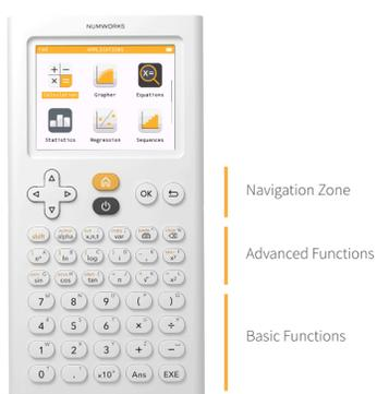
In the bottom section, you will find basic operations and the number pad. Notice that there is only one minus key. Here you will also find the  $\text{Ans}$  key which allows you to use the most recent result in your calculations. To compute a calculation, press the  $\text{EXE}$  key.
